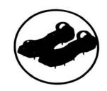
It is possible to completely coat the deck area with UPC Product #572 (Tan) before you start broadcasting sand onto it. In order to do this, you must wear nail shoes shown (golf shoes will work) to be able to walk on wet coating safely.
